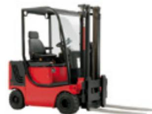
**M700-4 EEx** Electric 4-wheel counterbalance forklift truck
