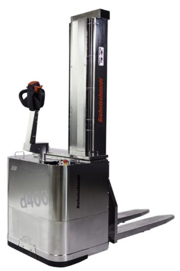
Since the use of stainless steel forklifts may not always be feasible due to their high initial cost, Sichelschmidt offers for these applications an optional low cost package "RR" for all pedestrian operated vehicles. This package may also be used in combination with explosion-proof fork-lifts for category 3GD (Zone 2/22) and 2GD (Zone1/21).
