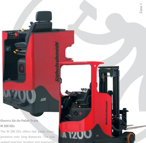
portation over long distances. The side seated operator position and ergonomic design offers a comfortable work environment for the driver. This 24V unit can be equipment with extended fork lengths, which enable you to handle multiple pallets at once. Power steering can be supplied on the 3G/3D models only. Equipping the M 200 EEx with tow hook, will transforms this unit into a high efficiency ride-on tow tractor
